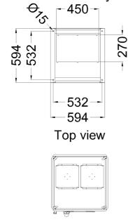
Bottom view ground fixing and cables entry
