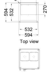
Bottom view ground fixing and cables entry
